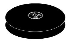
R-204 plastic spool, flange diameter 4.940", 16 mm x 200'. Square hole with two keyways and two offset round drive holes (each hole attached to keyway). Both flanges.\* 1.25" core diameter. Sp. 641.
