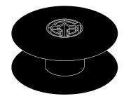
R-200 plastic spool, flange diameter 3.610", 35 mm x 100'. Side 1 – Square hole with three keyways and two offset drive holes. Side 2 – Square hole with two keyways and two offset drive holes.\* 1.265"core diameter. Sp. 425.
